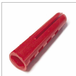
Red Plastic Rawl Plugs. Drill Size: 5.5/6mm, Screw Size: 6/8/10G
