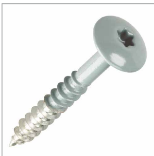
Grey coloured top stainless steel torx head self-tapping screws. Size: 11.5mm Ø head x 4.8mm Ø x 25mm.
