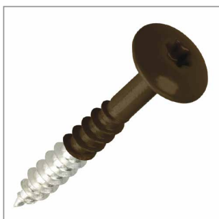
Brown coloured top stainless steel torx head self-tapping screws. Size: 11.5mm Ø head x 4.8mm Ø x 25mm.
