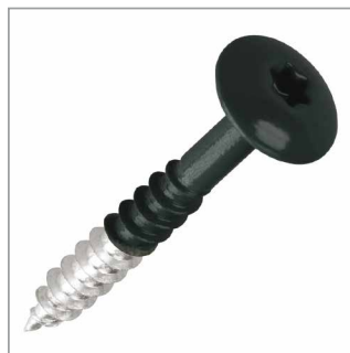
Black coloured top stainless steel torx head self-tapping screws. Size: 11.5mm Ø head x 4.8mm Ø x 25mm.
